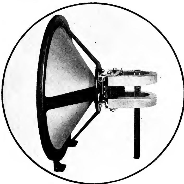
View of an inductor loud speaker motor with a paper cone attached. This loud speaker, of course, must be placed behind a baffleboard for best results.
